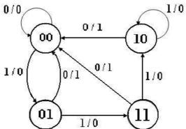
11. i). For the state below figure, design a synchronous sequential circuit using JK flip flops.
