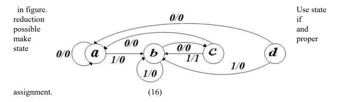
4. Derive the transition table, state table and state diagram for moor sequential circuit shown in below figure. (16)
